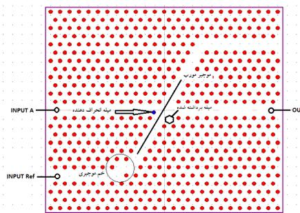
Figure 6 NOT logical gate structure
